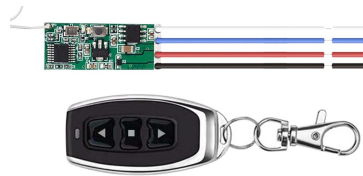
433 Mhz RF Wireless Transmitter and Micro Motor Control Module
