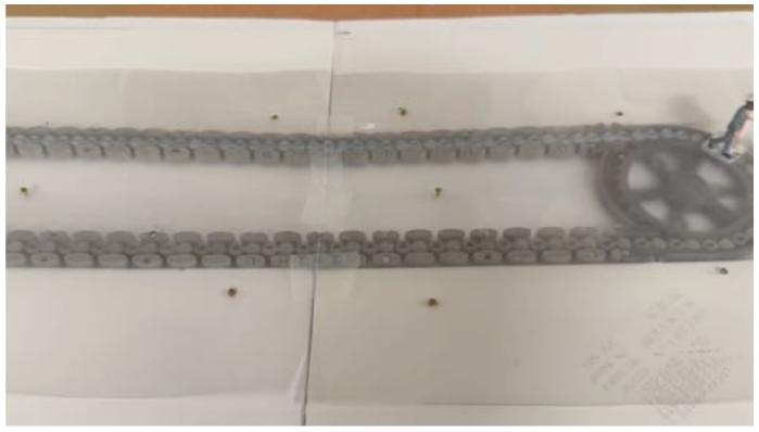
A small access space will need to present so the chain links can be separated.
