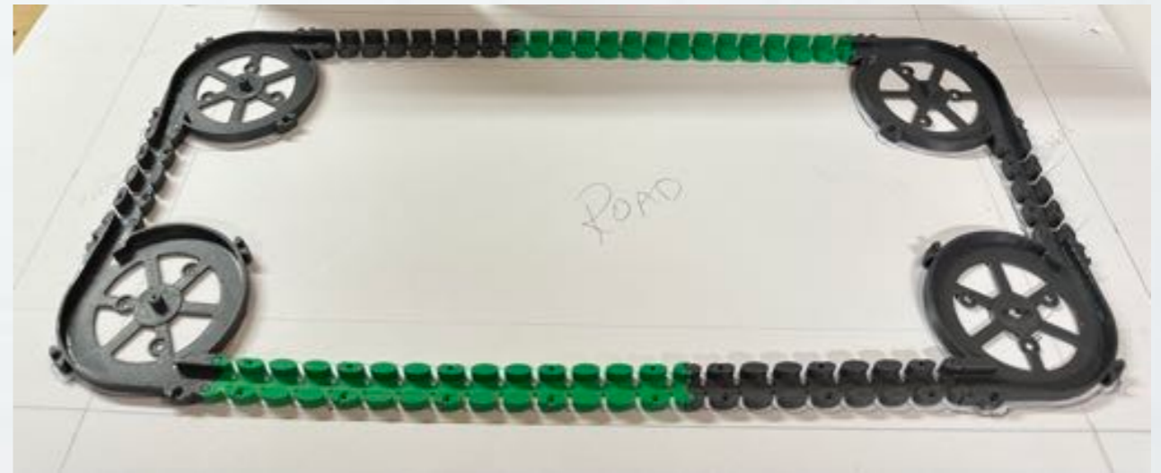
Track Components shown are early test prints, printed in-house using ABS filament on an FDM printer.
